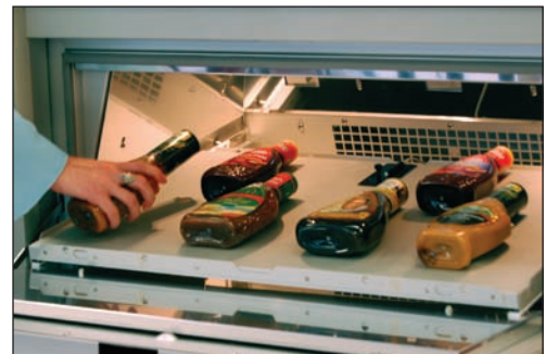
3-D specimens can be placed directly on the specimen tray and in most cases do not require a specimen holder.
