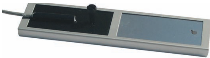
The Black Panel Temperature sensor is mounted in a 2x4" specimen holder.
