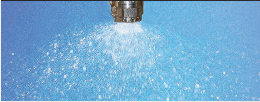
The Q-Sun uses a pure water spray to simulate outdoor moisture attack.
