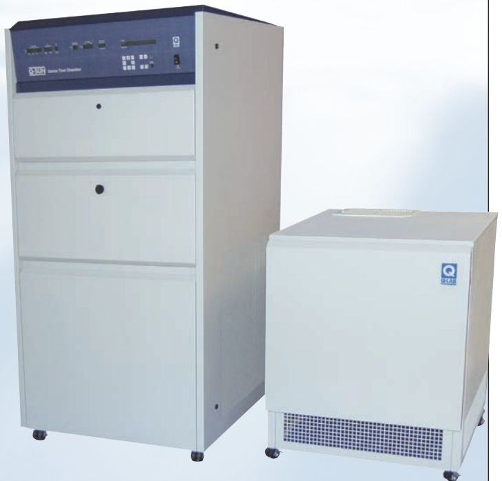
The chiller for the Q-Sun Xe-3 is a separate unit that sits next to the tester. The Xe-1's chiller serves as its stand.
