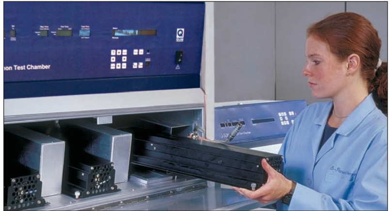
Q-Sun air-cooled lamps are easily accessible from the front of the tester.
