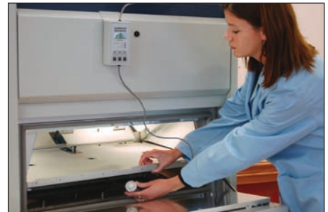
The CR20's UV sensor is placed into the calibration port located in the specimen tray.
